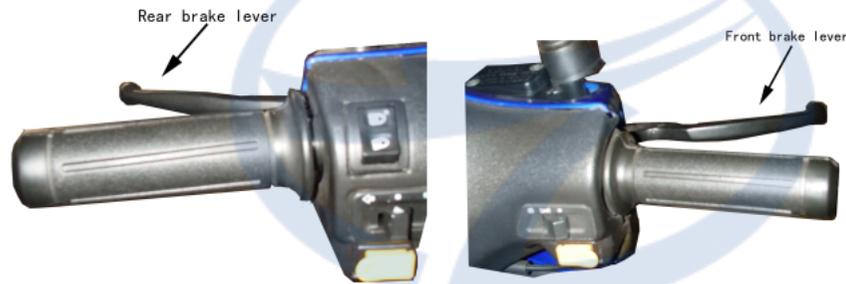
1. Squeeze the brake levers after quick returning the throttle bar.
